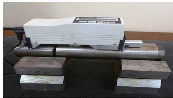
Figure 7. Roughness (Ra) was evaluated using a Mitutoyo SJ-301 portable tester
