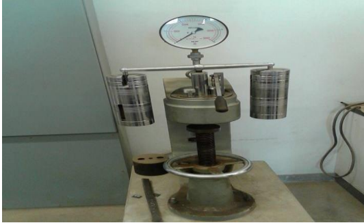
Figure 6. Surface hardness was measured using a Rockwell C (HRC) tester
