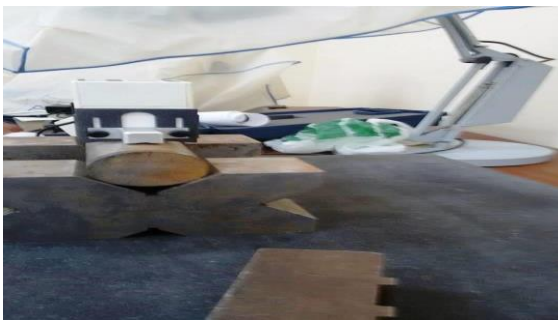
Figure 7. Roughness (Ra) was evaluated using a Mitutoyo SJ-301 portable tester
