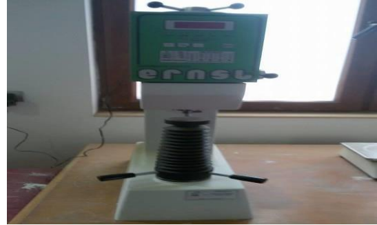
Figure 6. Surface hardness was measured using a Rockwell C (HRC) tester
