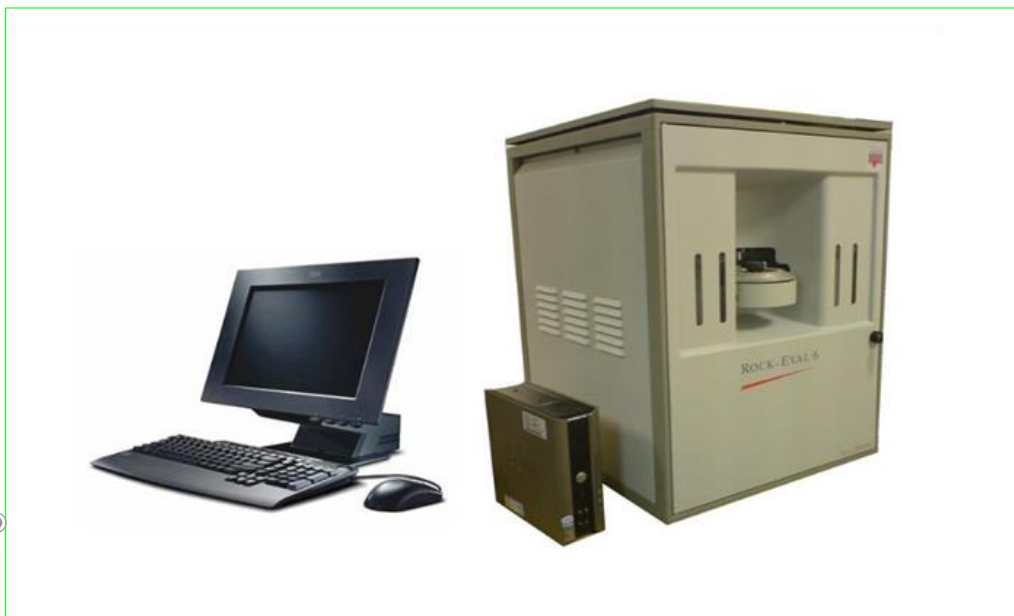
Figure 2. Illustrative picture showing the Rock-Eval 6 apparatus All these parameters are explaining and interpreting in Table (1).
